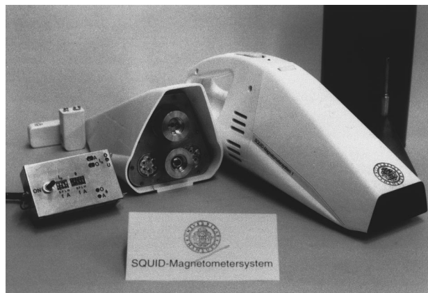
FIG. 1. Hand-held SQUID magnetometer system used for biomagnetic measurements. The cryostat can be seen in an additional front part shown in the middle. The complete system is depicted at the right side.
